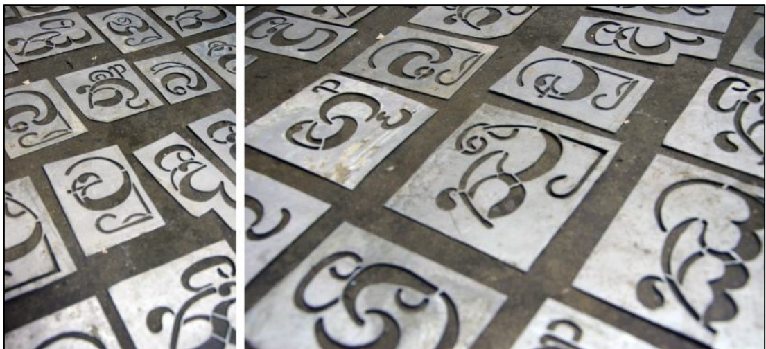
Figure 3.22: Stencils of Chithra used for the Shadowgraph machine
